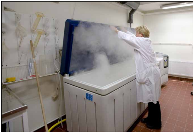
Figure 1 – Salt spray chambers create test conditions that are rarely, if ever, observed in practice.
