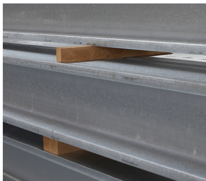
Fig 2. Example of use of spacers to ensure a free-flow of air to enable drying
