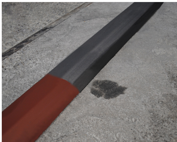
Fig 3. Use of an anti-galvanizing paint solution as a masking system
