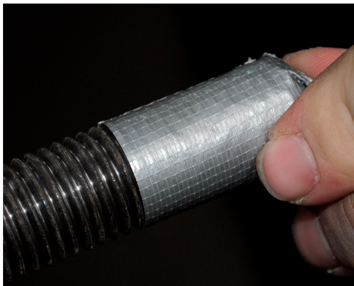
Fig 1. Masking with fabric tape prevents a galvanized coating
