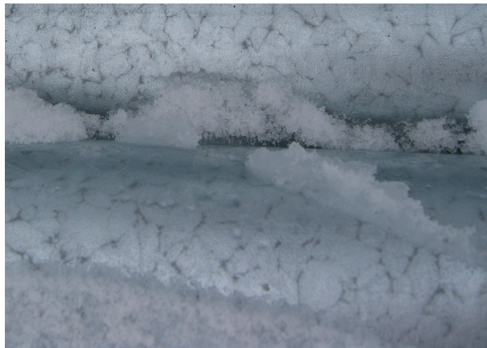
Fig 3. Grey cellular appearance of the zinc coating
