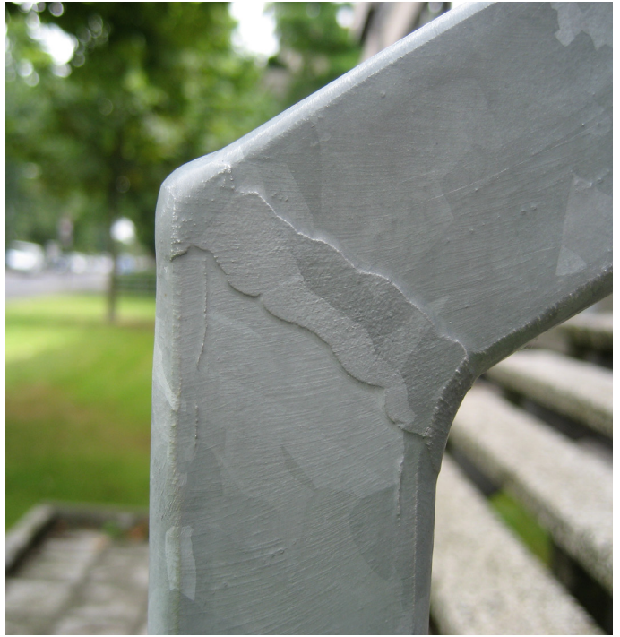
Fig 4. A weld that was ground flush prior to galvanizing. The high silicone content of the weld metal has then led to a thicker coating forming locally
