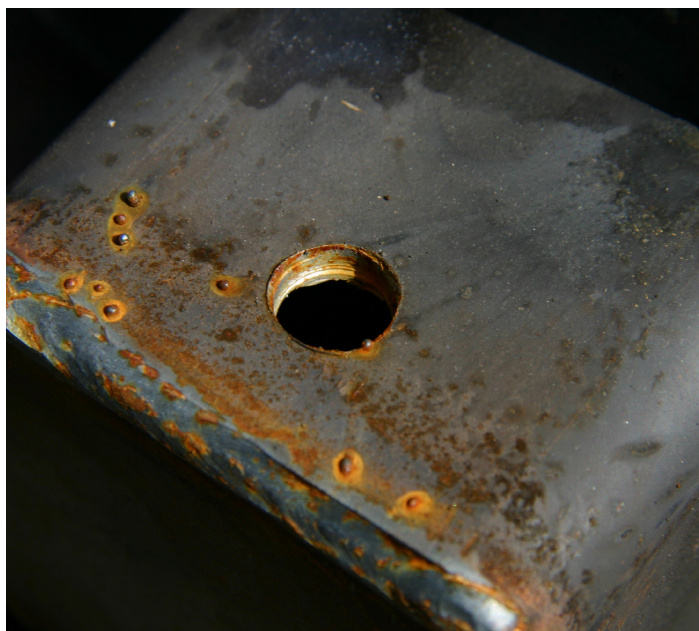
Fig 1. Weld spatter present on steel before galvanizing
