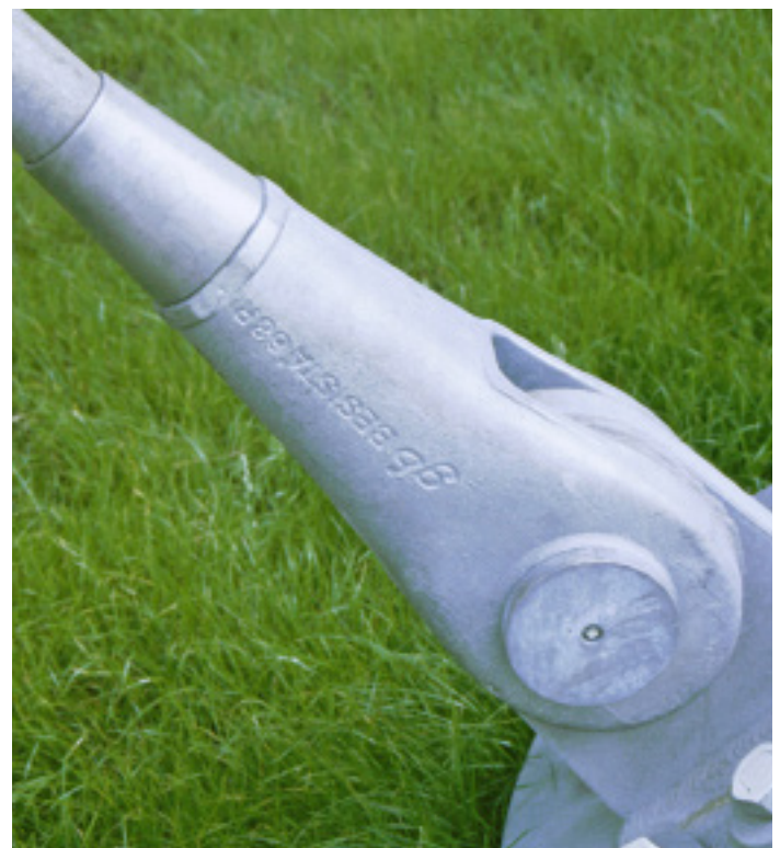
Fig1: 'A hot dip galvanized casting'
