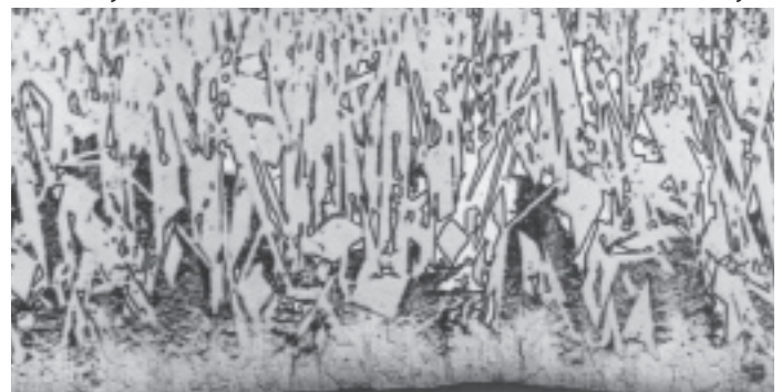
Fig 3. Microstructure of a thick coating obtained on a reactive steel
